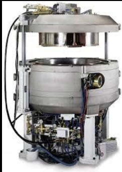
Cyclotron for production of short-lived radionuclides (C11, F18)
